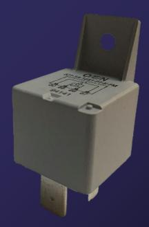
Rated for 100A@12VDC or 50A@24VDC. Available in 1 Form A configuration
