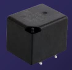
Rated for 45/30A@12VDC or 20/10A@24 VDC. Available in 1 Form A, 1 Form C configurations
